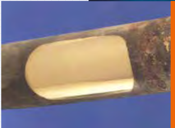
The image is an example of Tungum Tubing after 10 years at sea on a dredger. Only the grime and oxide coating has been removed from the tube exterior.
